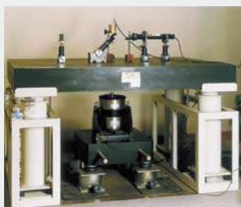
Absolute calibration setup for vibration accelerometers
